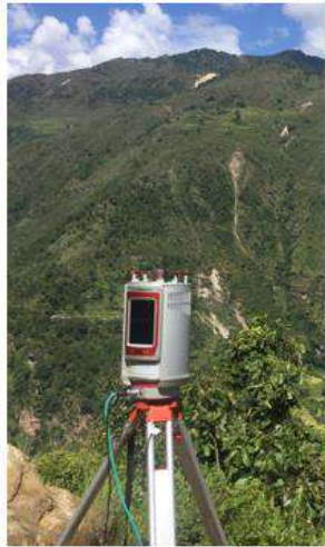
Terrestrial Laser Scanning
