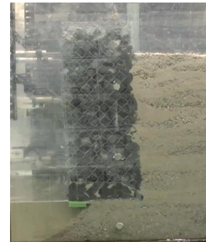
Collapsed foundation ground
