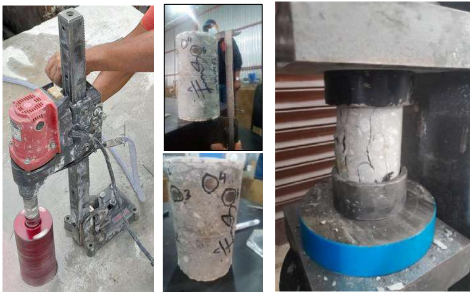
Figure 2: Core cutting, measurement & testing
