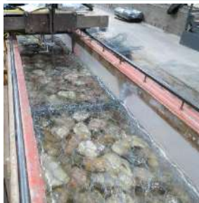
Effect of different stones (size & grading) and mattress configurations (diaphragm & spacing)
