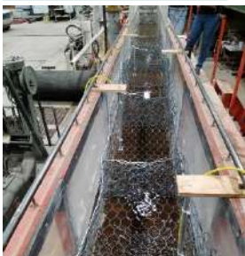
Effect of the mattress wire mesh (only)
