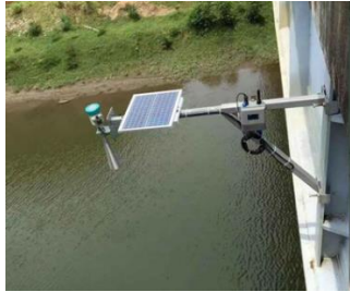
Flood and Rain Sensor, Datalogger
